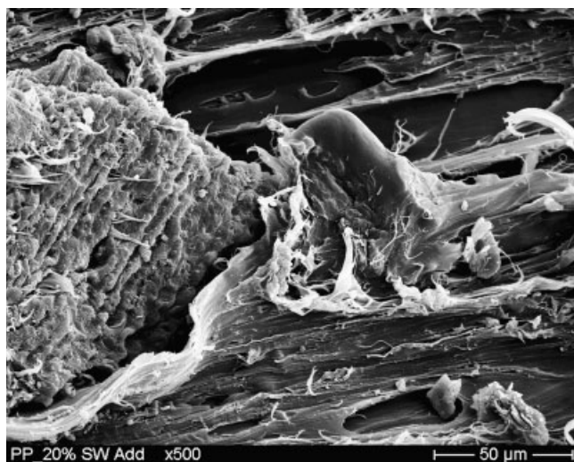
Figure 11 SEM micrograph of fractured specimen of seaweed PP composite SWAdd with TPE additive.
